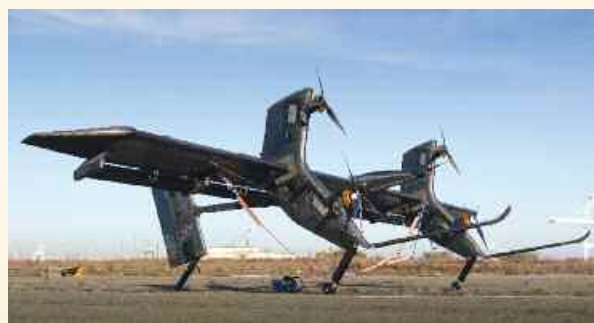
Makani Power’s 1-megawatt prototype airborne wind turbine weighs a fraction of a traditional 1-megawatt turbine.
